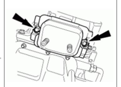
9. Loosen the bolt and disconnect the transmission vehicle harness connector.
