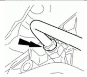
15. If equipped with dual generators, rotate the tensioner and remove the outer accessory drive belt from the crankshaft pulley.
