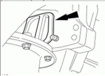
17. Remove the steering dampener-to-frame bolt and nut and position the steering dampener aside.
