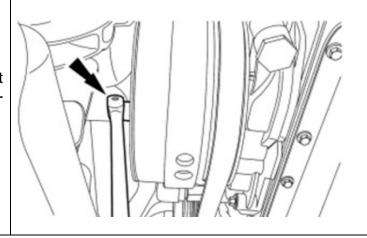
19. Remove and discard the 8 torque converter-to-flexplate nuts.
